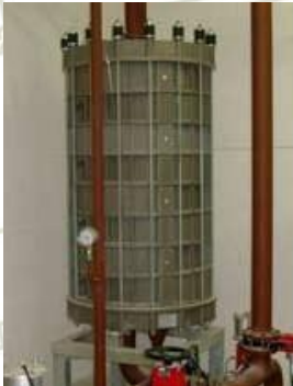
External heat exchanger
