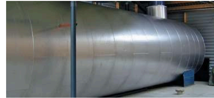
Horizontal/Plug flow digester
