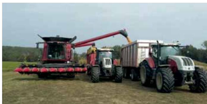
Unloading of grain and cob tanks at the same time. Source: CREA-IT
